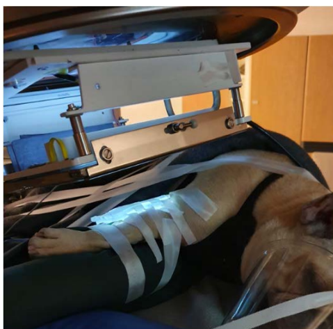
Figure 1: Treatment setup for the first patient receiving FLASH-RT at our clinical linear accelerator.
