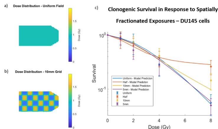
Figure 1: Example dose distributions for the (a) Uniform field and (b) 10 mm grid pattern exposures where the mean dose delivered to each T25 flask is 1 Gy. (c) The clonogenic survival resulting from each of the plans at the 1, 2, 4 and 8 Gy dose points is compared to the predictions made by the mathematical model.
