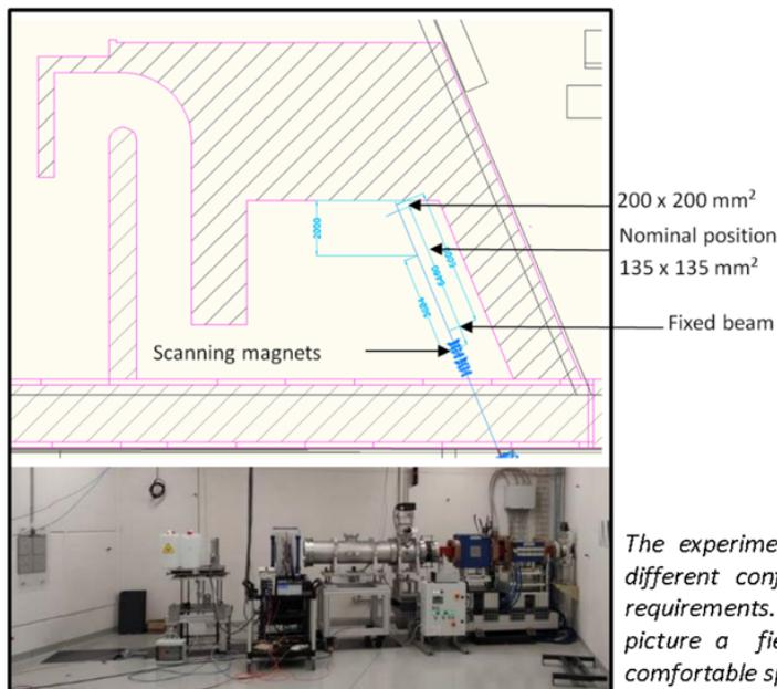
The experimental room at CNAO can be arranged in different configurations according to the experiment requirements. In the nominal configuration shown in this picture a field of 135 x 135 mm<sup>2</sup> is available with comfortable space around the irradiation position.
